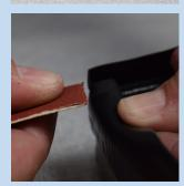
2.2 Roughen the glued areas with sandpaper. *Tip* Roughening improves the adhesion.
